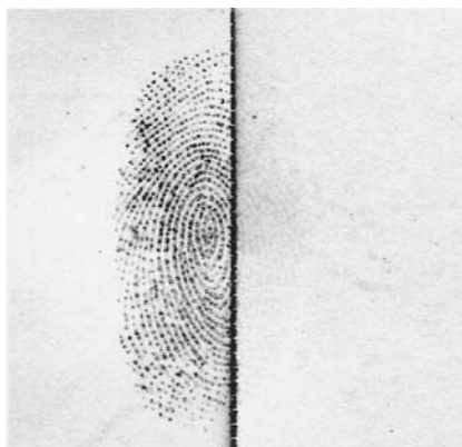
FIG. 4—Ninhydrin-treated print: right half of the print was kept in ESDA humidifier for 60 min prior to fingerprint process.
